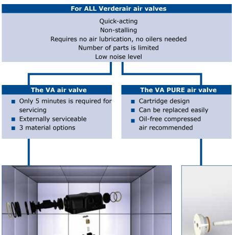
The Verderair VA series is equipped with an air valve that has a modular cup and plate design. This air valve design is based upon the existing model used in Verderair pumps for many years, but is now re-engineered to be the most efficient one.
