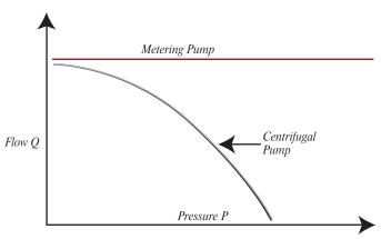
2. Unlike centrifugal pumps, flow rate is not greatly affected by changes in discharge pressure.
