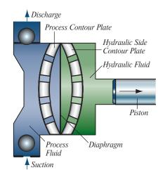
Traditional Liquid End with Process and Hydraulic contour Plates (refill system not shown)
