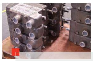
Our patented PCR® heat exchanger is the industry-leading solution for refrigerant air dryers. Featuring a 3-in-1 design, these units offer energy-saving heat recovery between the incoming and outgoing air streams, an efficient refrigerant cooling section, and integrated moisture separation all in a single, compact, cost-effective package.
